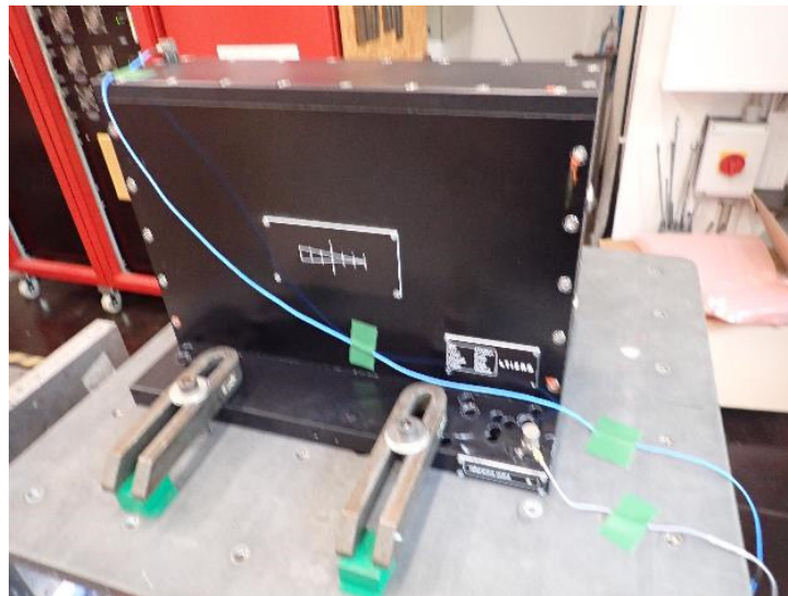
Figure 3 — Reference specimen mounted on a vibration test system with clamp-type fixation, illustrating a configuration identified as a primary source of inter-laboratory result divergence. The compliance at the fixture–table interface directly affects control-loop behaviour at specimen resonance frequencies.
